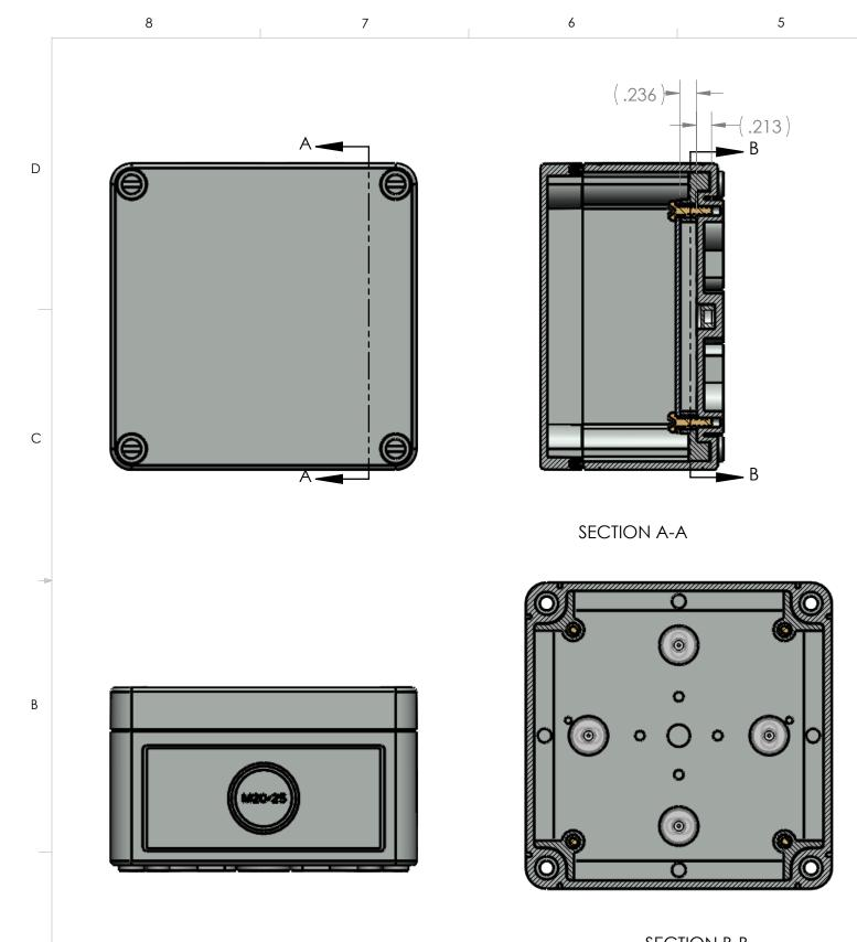
BOM Table ITEM NO. PART NUMBER QTY. Rev. Description SK-14-02 SK-14B-02 BASE COVER SK-14C-02 .2 1.3 SK-KIT-03 HARDWARE KIT 1.3.1 SCREWS-014 ASSEMBLY FASTENER 4 1.3.2 SK-CAP-02 SCREW HEAD CAP MOUNTING PLATE KIT SK-14K SK-14P MOUNTING PANEL SPACERS WITH RUNNER 2.2 SK-97S 2.2.1 SK-97S-02^SK-97S **CAPTIVE BOSS** 2.2.2 CORNER BOSS SK-97S-01^SK-97S 2.3 SCREWS-024 M3.85x1.8 SPAX X 13mm, PAN HEAD, PHILLIPS/SLOTTED
