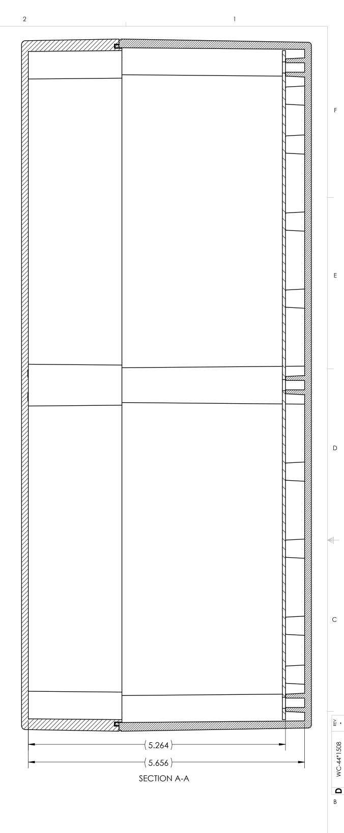
NOTES: 1. ENCLOSURE DESIGNED TO NEMA 1, 2, 4, 4X, 12, 13. 2. UL LISTED TO UL508-4X SPECIFICATIONS (UL FILE E194432). 3. SERVICE TEMPERATURE: -40°C TO 120°C
