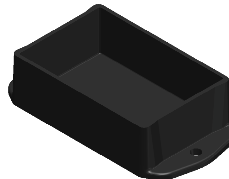
BX-2310BXX: BX SERIES BASE, BLACK, WITHOUT MOUNTING BOSSES MATERIAL: ABS FLAME RATING: UL94V-0
